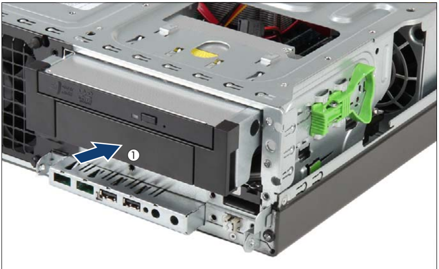
Figure 61: Installing the 5.25-inch ODD/HDD bracket with the slimline ODD
